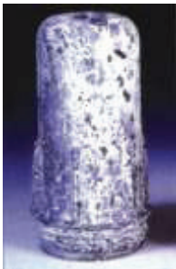
Rapid corrosion of untreated aluminium
