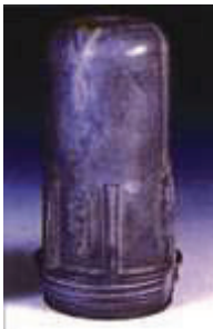
No corrosion with Alocrom treatment
